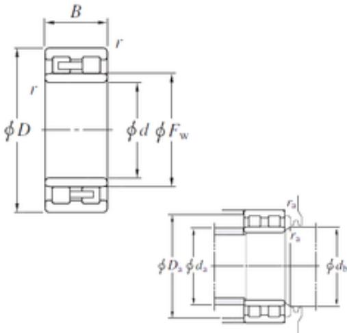
NNU3144 Bearing 2D drawings and 3D CAD models
